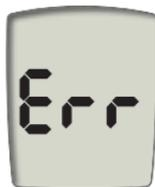
There was not enough blood on the test strip to start the test. Repeat the test with a larger drop of blood.
