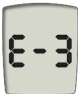
The meter is having trouble reading the code key. Take the orange code key out and put it back in again. For help, see Chapter 1, "Coding the Meter."
