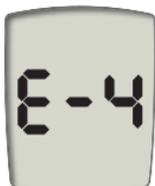
There is a problem reading the test strip. Clean the test strip guide (see Chapter 5, "Cleaning Your Meter") and make sure the test strip is straight when you re-insert it.
