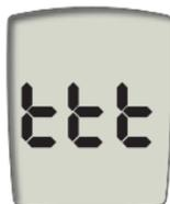
The temperature is above or below the proper range for the meter. Move to an area between 50°F and 104°F, allow the meter to warm up or cool down slowly to room temperature and repeat the test. If you get a result with a temperature icon, it could be inaccurate. Do not artificially heat or cool the meter.
