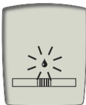
5. When you see the flashing blood drop, hold the lancet device against the side of your fingertip and press the release button.
