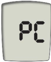
When “PC” flashes on the display, you have 2 minutes to start transferring data before the meter shuts off.
