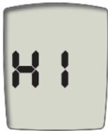
Blood sugar is higher than the measuring range of the system. See Chapter 3, "Understanding Your Test Results."
