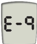
The test strip was not inserted correctly, it was removed during testing, or blood was applied too soon. Repeat the test with a new test strip. Make sure you insert the test strip until the arrowheads are no longer visible, with the orange square facing up (see Chapter 3, "Running a Blood Sugar Test").
