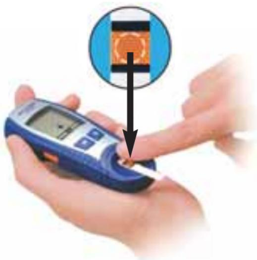
7. Touch the blood drop to the center of the square orange pad. Do not bend the test strip.
