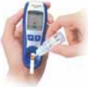
3. When the flashing blood drop appears on the screen, press **S** to mark the test as a control. You can also do this right after you get your test result, but not after the meter turns off. A control bottle symbol is displayed on the screen and stored in the memory to show that this result is from a control test.
