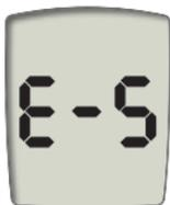
There is a problem reading the test strip or the test strip is used, dirty, or expired. Clean the test strip guide (see Chapter 5, "Cleaning Your Meter") and repeat the test with a new test strip.
