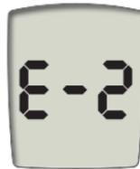
The wrong code key is in the meter. Put in the orange code key that came with the container of test strips you are using.
