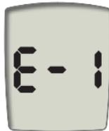
The test strip is not inserted correctly. Make sure the arrows are pointing toward the meter and the orange square is facing up and is positioned over the measuring window.
