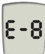
The code key is defective or not inserted correctly. Take the orange code key out and put it back in the meter (see Chapter 1, "Coding the Meter").
