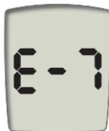
A test error has occurred, or there is electromagnetic interference. Repeat the test. If you get the same message, move away from sources of interference and repeat the test.
