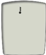
The temperature is above or below the proper range for the meter (50°F to 104°F). Move to an area between 50°F and 104°F, allow the meter to warm up or cool down slowly to room temperature. Do not artificially heat or cool the meter. Refer to "Proper Testing Conditions," Chapter 3.
