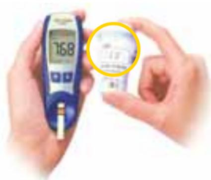
1. With the meter off, slide the orange code key into the code key slot. It should easily snap into place.
