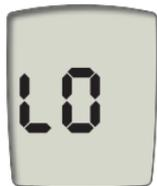
Blood sugar may be lower than the measuring range of the system or the test strip has been bent. See Chapter 6, "Specifications." We recommend retesting your blood sugar according to Chapter 3, "Testing Your Blood Sugar." Verify results by running a control test. See Chapter 2, "Running a Control Test."
