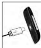
Plug the small end of the USB cable into the meter.
