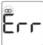
The meter was unable to pair with a mobile device.
