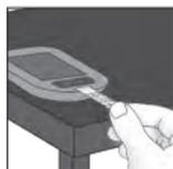
Insert the metallic end of the test strip into the meter. Place the meter on a flat surface.
