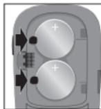
Slide the new batteries under the black tabs with the **(+)** side facing up.
