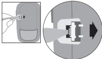
Open the child-resistant battery door by inserting a narrow object, such as a pen, into the slot (see image above). Push the tab in the direction of the arrow and lift the battery door up.
