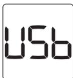
The meter is connected to a PC and a blood glucose or control test cannot be performed.
