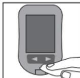
Turn the meter off and wipe the entire meter surface with a Super Sani-Cloth. Carefully wipe around the test strip slot and other openings.
