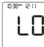
Blood glucose may be lower than the measuring range of the system (lower than 20 mg/dL).
