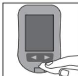
Turn the meter off and wipe the entire meter surface with a Super Sani-Cloth. Carefully wipe around the test strip slot and other openings.
