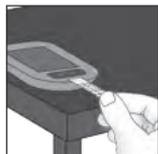
Insert the metallic end of the test strip into the meter. Place the meter on a flat surface.
