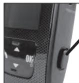
Press here to eject test strip
