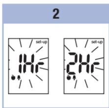
Press and release ① repeatedly until set-up and the flashing 1Hr or 2Hr appear on the display.
