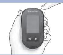
Press and release ① (power/set button) to turn the meter on.
