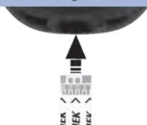
Insert the test strip into the meter in the direction of the arrows.
