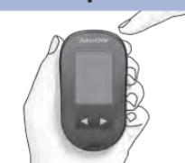
Press and release ① to turn the meter on.
