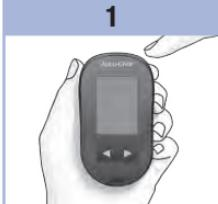
Press and release ① to turn the meter on.
