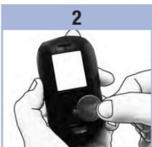
Remove the old battery and place the new one in the meter with the (+) side facing up.
