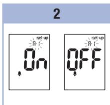
Press and release ① repeatedly until the bell symbol, **OFF**, **set-up**, and the flashing **A-1** appear on the display.
