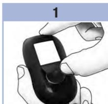
Push the tab in the direction of the arrow to open the battery door on the back of the meter.
