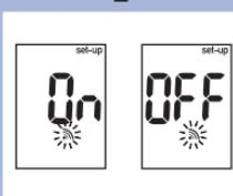
Press and release ① repeatedly until the flashing beeper symbol and On or OFF appear on the display.
