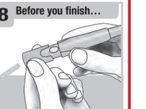
Remove the lancing device cap. Point the lancet away from you. Slide out the ejector to release the lancet.
